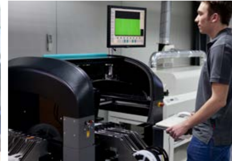
Platinen-Bestückung / LED automatic placement machine
